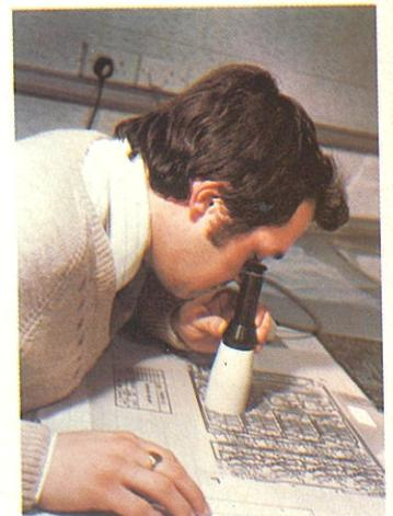
A development engineer at GEC Telecommunications Ltd checks artwork against a computer-aided design for a printed circuit board which will be used in a private telephone exchange.
