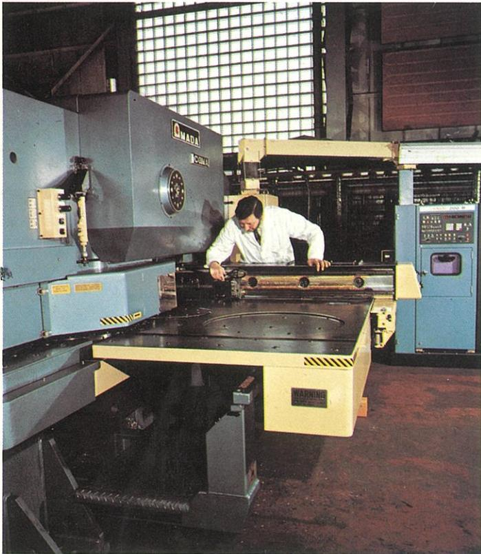
A new, fast turret punch installed in Keith Blackman Ltd's new factory at Rugby. The punch produces components for Keith Blackman's new ranges of centrifugal fans and dust filters.
