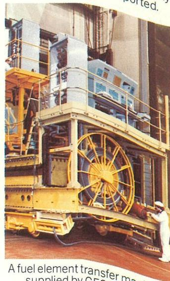
A fuel element transfer machine supplied by GEC Reactor Equipment Ltd to Wylfa nuclear power station. The machine holds 64 fuel elements.
