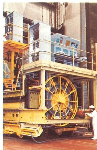
A fuel element transfer machine supplied by GEC Reactor Equipment Ltd to Wylfa nuclear power station. The machine holds 64 fuel elements.
