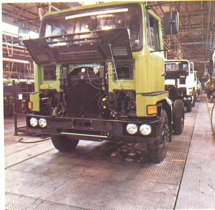
Lorries travelling on a flush floor slat conveyor system supplied by GEC Mechanical Handling Ltd in use at Vauxhall Motors, Dunstable.
