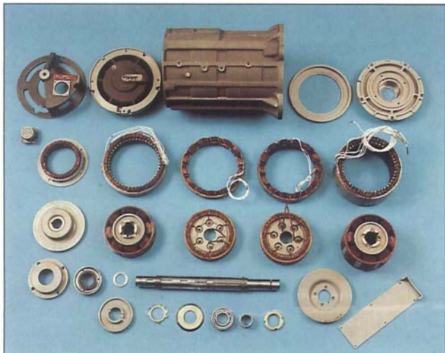
Machine and wound components, manufactured in-house at Titchfield for the Spearfish electrical alternator.
