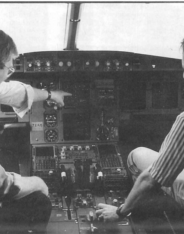
Field Service Engineers discussing the Slats and Flaps control system on an Airbus A320.
