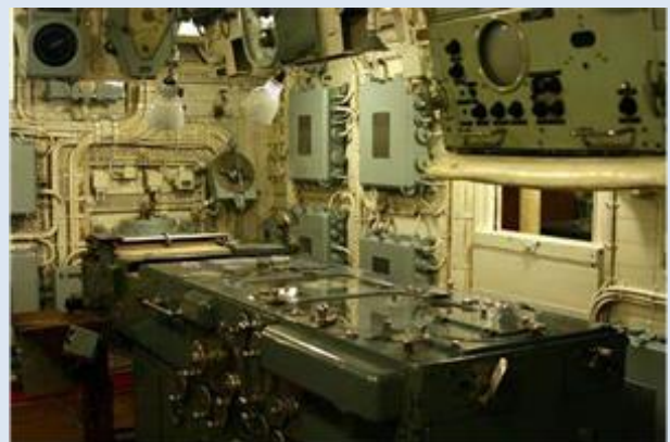
The picture below is of the Fire Control Table in HMS Belfast.
