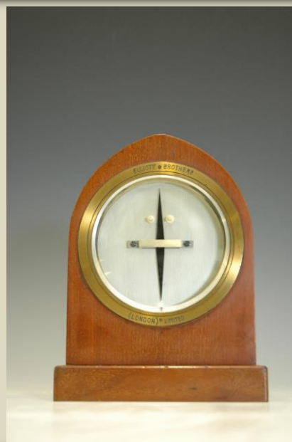
Telegraph Galvanometer, by Elliott Brothers (London) Ltd., 20th Century Courtesy of The Museum of the History of Science Oxford.
