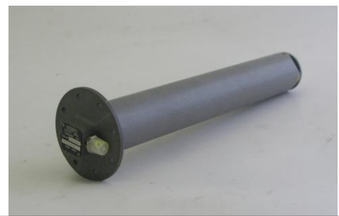
Fuel Level Tank Sensor Unit from a Vickers Viscount around 1967
