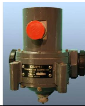
Fuel Flow Transmitter from a Wessex Helicopter around
