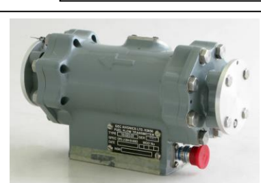
Twin Fuel Flow Rate Indicator for the Tornado around 1973
