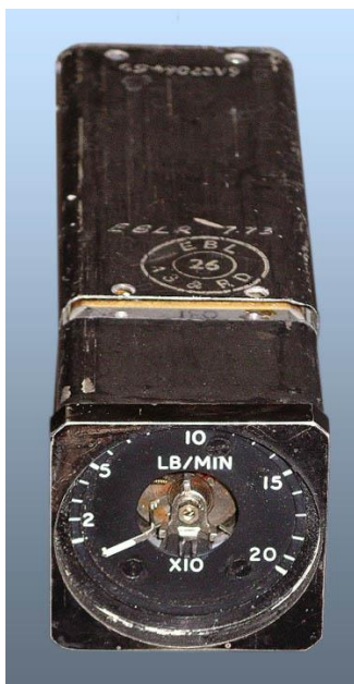
Fuel Flow Rate Indicator supplied for the Trident around 1968
