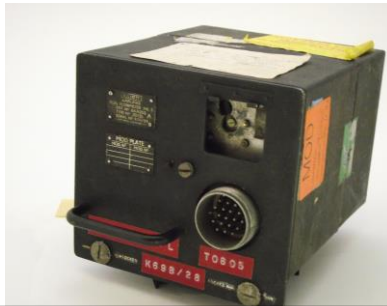
Fuel Flowmeter Amplifier from a Vulcan around 1958
