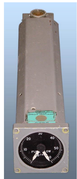
Twin Fuel Flow Rate Indicator for the Tornado around 1973
