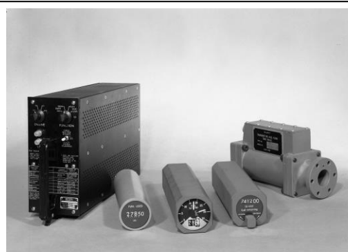
Fuel Flow system supplied for Concorde around 1970
