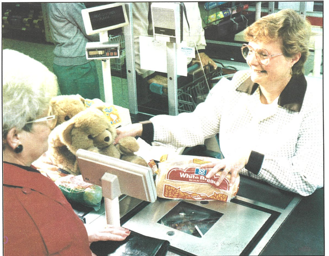
The scanner scale allows fast throughput of fresh products across the checkout surface. Goods are weighed in front of the operator instead of being lifted onto a separate scale.
