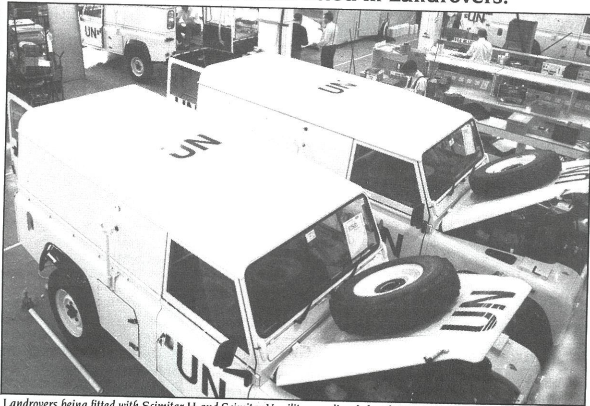
Landrovers being fitted with Scimitar H and Scimitar V military radios, before being shipped to Bosnia.
