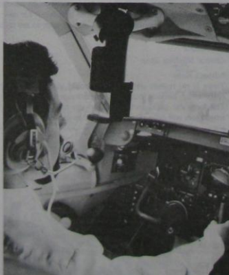
The Marconi Avionics MONOHUD, fold away head-up display, originally developed for use in airliners as an aid to safer landing and take off, is now also being offered for use in military helicopters. Like other head-up displays, MONOHUD makes an ideal sighting and weapon aiming instrument, an important factor in many kinds of military helicopter.
