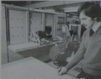
The picture, one of the first of the LF ATE to be generally released, shows the LF ATE being checked out with a TORNADO unit under test. At the controls is Carol Finch, Confidential Secretary, learning that operation of this advanced equipment has much in common with other keyboard equipment found in the modern office. In the foreground is Esmond Good, Commissioning Engineer.
