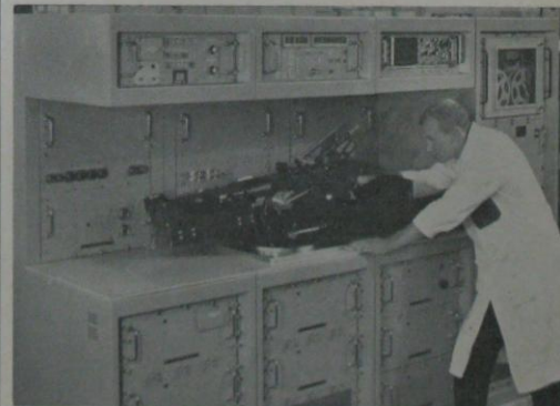
A head-up display mounted for testing in the first SSE console before it left for the USA.
