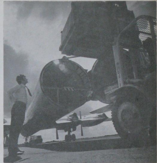
Mike Kitley, who has since left ATED, supervises the loading of the first SSE through the swing tail of CL-44 turboprop cargo aircraft in which it was flown to Dallas, Texas.
