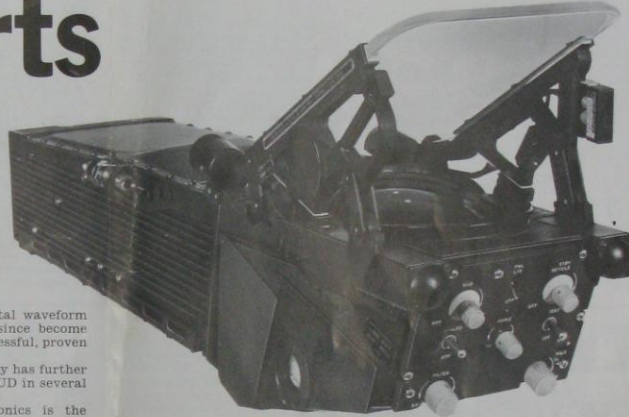
Head-up display Pilots Display Unit and electronics unit supplied for A7 Corsair
