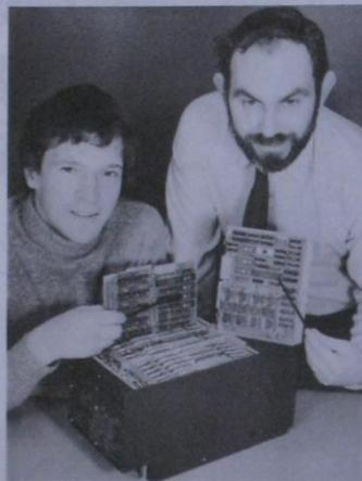
Two of the engineers in the Company's Flight Controls Division who are closely involved with the A310 slat and flap control system are (right) Geoff Holland B.Sc., C.Eng., M.I.E.R.E. who is pointing out one of the Fairchild 6800 microprocessors used in the system, Anthony Brown B.A., B.A.I. (left) is indicating the other, an Intel 8085.
