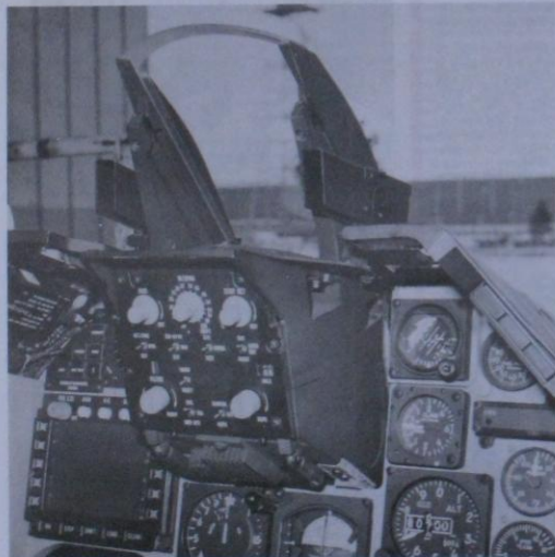
The Marconi Avionics head-up display is a central feature in the cockpit of the General Dynamics F-16 fighter. In use throughout every phase of flight, it provides the pilot with information for piloting, navigating and weapon aiming.
