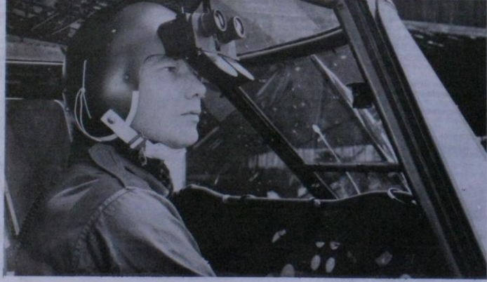
The prototype helmet mounted night vision system for pilots.
