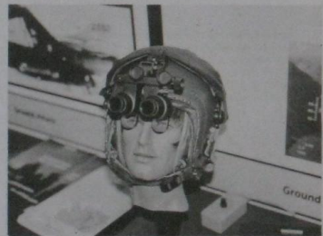
This improved low weight version of the GEC Avionics "Cat's Eyes" night vision goggles gives pilots the ability to see in the dark without affecting the normal cockpit instrument scan as has been proven in a series of 78 night vision and attack trials in a TA-7C aircraft at China Lake, California. They are also the only night vision goggles available which enable a pilot to see FLIR imagery and flight symbology on any head-up display, including the wide angle systems with diffractive (holographic) optics.
