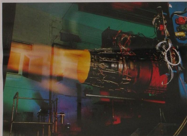
The EJ200 full scale development engine undergoing Reheat trials at Rolls-Royce, Bristol. (Picture by courtesy of Rolls-Royce plc.)
