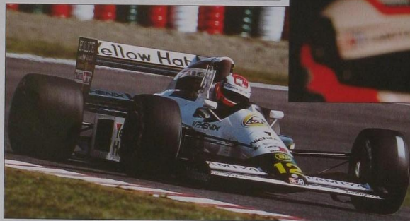
The Team Lotus Formula One car. Inset is the miniature eyepiece which is mounted inside the driver's helmet at the lower rim of the vizor aperture. (Courtesy of Team Lotus).
