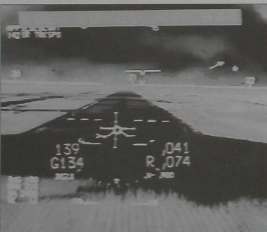
Sequential stills from a cockpit video of an EVS/ILS approach using the new system. The runway approach lighting is switched off.
