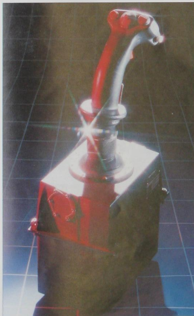
The Advanced Side Stick Controller for the American YF-22A Advanced Tactical Fighter is used in the cockpit Demonstrator, out of view in the picture above.
