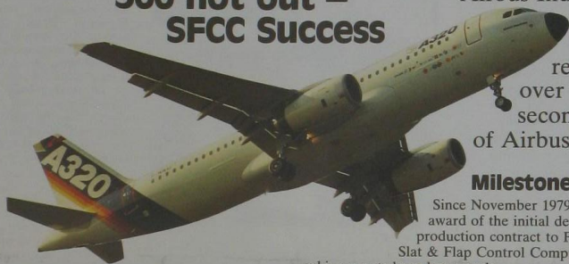
The A320 in landing configuration with the FCD-controlled flaps and slats deployed.
