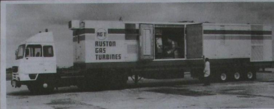
The new Ruston Nomad mobile generating set.
