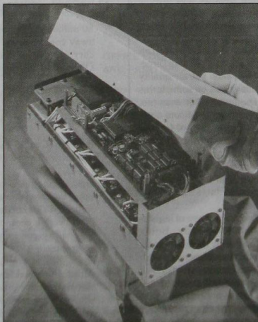
The Marconi Controller is ten times smaller than conventional motor controllers.
