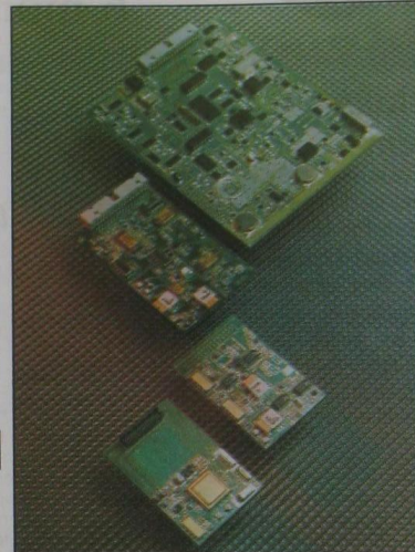
WLAN technology from GPS. From top to bottom, the progressive integration of the radio transceiver. The final version has space for system protocol circuitry.
