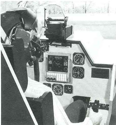
The cockpit which "hears and obeys" – FARL's direct-voice input developments
