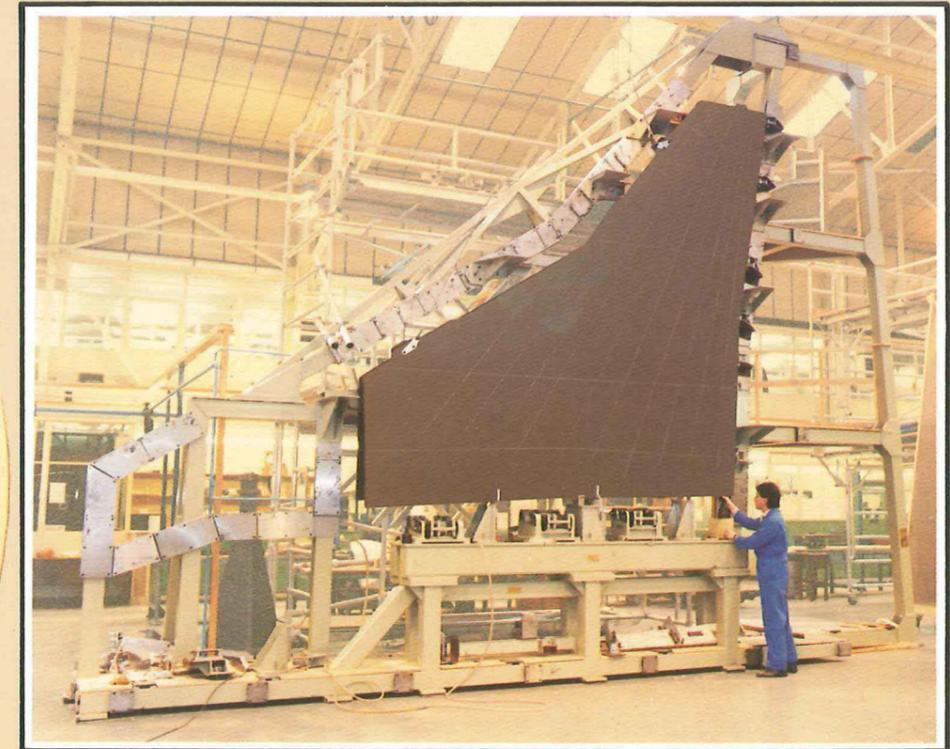
4. The co-bonded structure, having been erected in its assembly jig, is mated with the upper skin for initial fitting trials.
