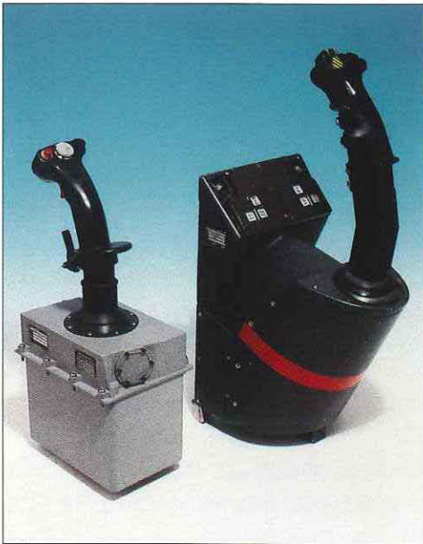
The side stick designed for the YF22 with the centre stick for the EAP.
