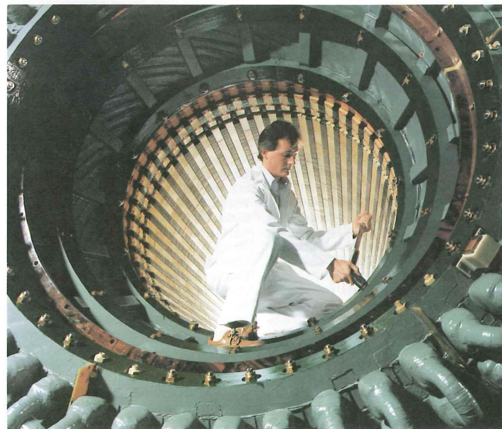
Works assembly of the stator for a standard large generator.
