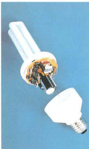
OSRAM-GEC's new Opus EL lamp. Picture reveals the control mechanism of this new fluorescent lamp which can be used to replace a tungsten lamp without the need for a special fitting. The new lamp uses less electricity and lasts longer than today's popular electric light bulbs.
