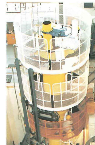
One of four plug unit handling machines designed and built by GEC Energy Systems for use in advanced gas-cooled reactor power stations.
