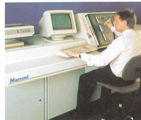
MIDATA 590 automatic test equipment from Marconi Instruments is used by computer, telecommunications and defence manufacturers for testing complex printed circuit boards.
