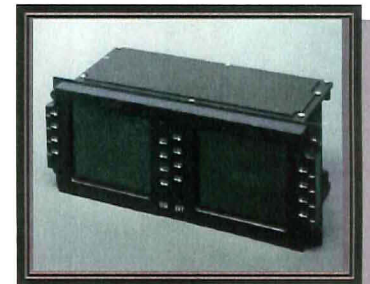
Display Avionics Management System
