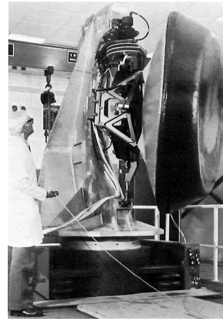
A development model of the AEW Aerial and Scanner undergoing vibration tests
