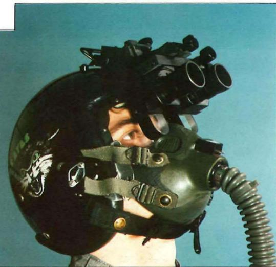
"Cat's Eyes" NV goggles permit night vision outside the cockpit and a capability to read normally lit instruments.
