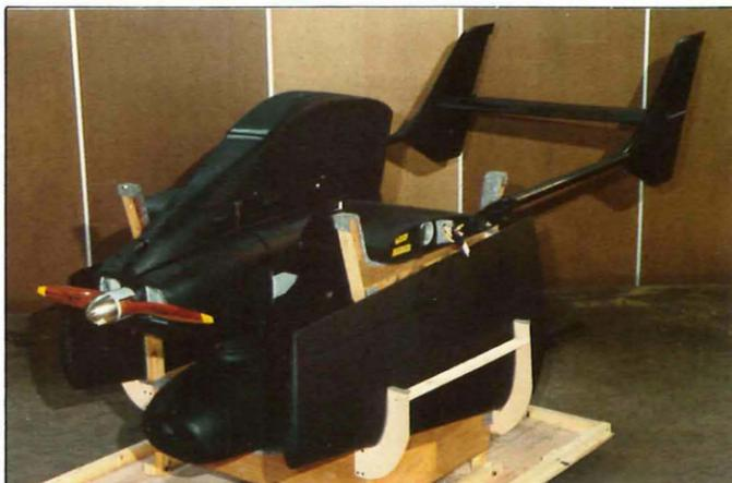
GEC Avionics is the prime contractor for the British Army Phoenix Remotely Piloted Vehicle and surveillance system.
