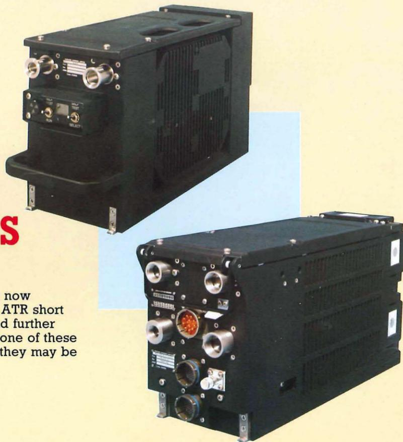
Single and dual channelled ADC's are now available which have 1/4, 3/8 and 1/2 ATR short chassis, suitable for rack mounting, and further options for direct surface mounting. None of these ADC's require forced air cooling and they may be powered from AC or DC sources.
