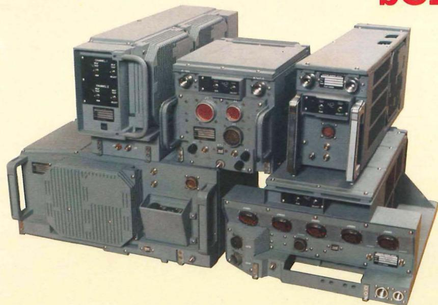
SCADC (Standard Central Air Data Computer) program uses a core set of standard Air Data Computer modules which can be packaged to satisfy air data computing requirements for any aircraft. The 35 aircraft variants being updated by the USAF and USN in the SCADC program are retrofitted by only 5 SCADC variants.
