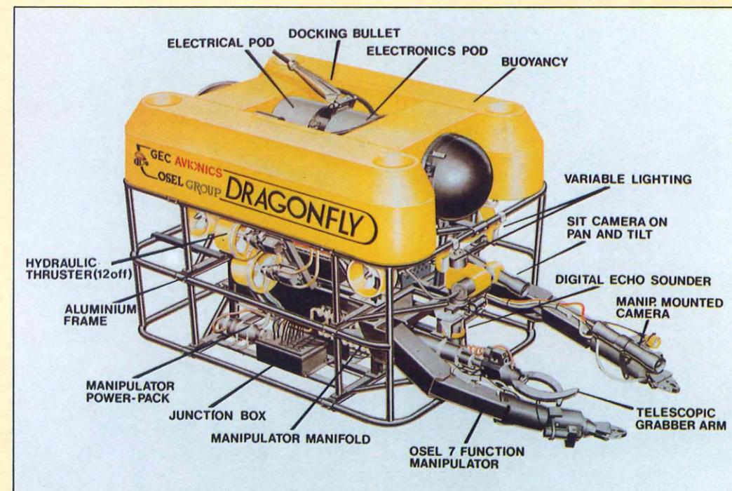
Another product of the Offshore Projects Group is Dragonfly, which has been developed jointly with OSEL, Gt. Yarmouth. Dragonfly has been designed and constructed to provide a truly modular facility for quickly and simply changing the payload of the vehicle. Dragonfly comprises of a base vehicle
