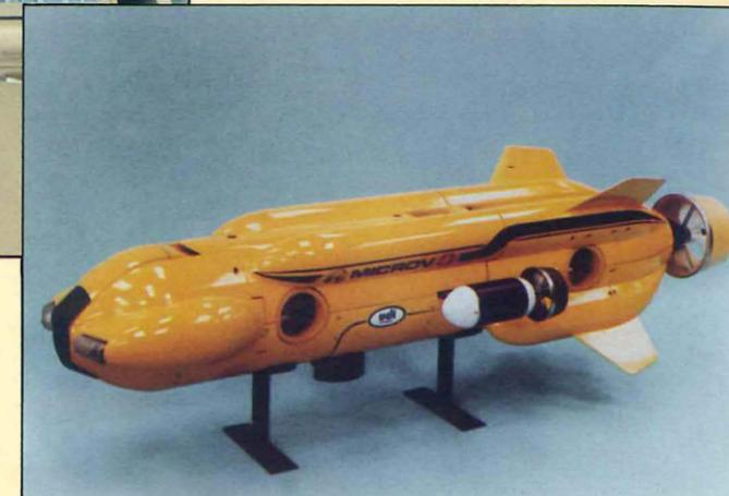
The Offshore Projects team of ISD (based at Nailsea) has developed MICROV — a fast, powerful and manoeuvrable inspection vehicle (Remotely Operated) which is equipped with Sonar and Viewing systems for use in the Offshore Oil Industry, and MIDAS a mine countermeasure ROV. ISD also manufacture subsea controls, incorporating new technologies such as 'touch screen' controls.
