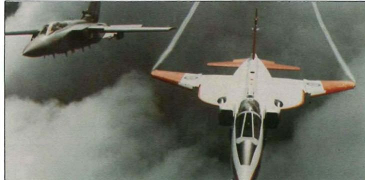
The BAE Jaguar depends on the GEC Avionics digital flight control at the heart of the aircraft's 'Fly-By-Wire' system for safe, stable handling.
