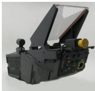
The dummy PDU fitted on the YF-16 first flight
