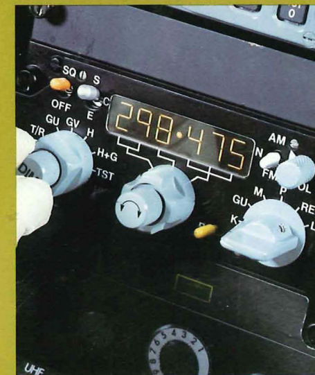
The AD3400 multimode communications system, adopted by British and overseas air forces, can cover all VHF/UHF bands, AM and FM.
