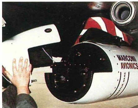
High-performance FLIR pods, based on inter-operable TICM II modules, equip subsonic and supersonic aircraft.
