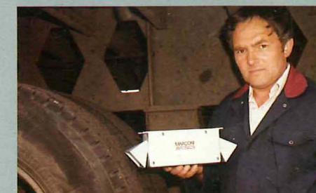
Doppler Velocity Sensor for road vehicles measures groundspeed by radio beams as in aircraft dopplers. Sensors have been supplied for magnetically-suspended train systems.
