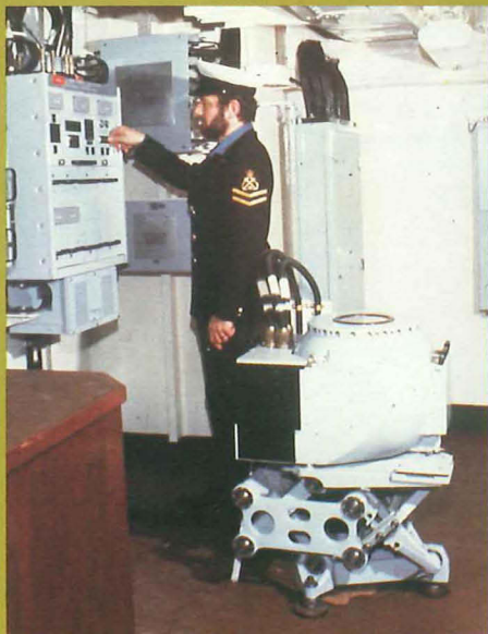
NCS-1 is the central heading and attitude reference for many naval vessels.
