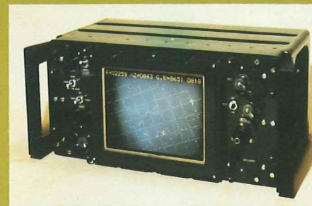
The FASTAR battlefield surveillance radar, successor to ZB 298, features a new easy-to-operate display of perimeter and target data.
