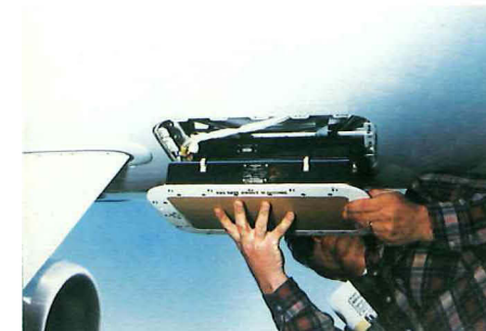
AD 660 Doppler Velocity Sensor, an effective groundspeed measurement system for airliners, can also be used in tactical navigation.
