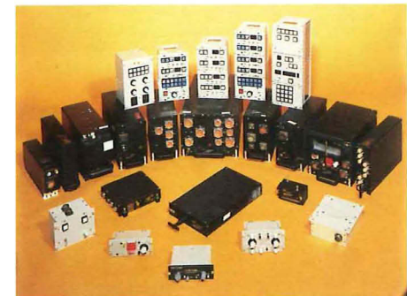
The Communications sub-system for AEW Nimrod aircraft provides clear and secure voice and data on HF, VHF and UHF for the Mission and Flight crews.
