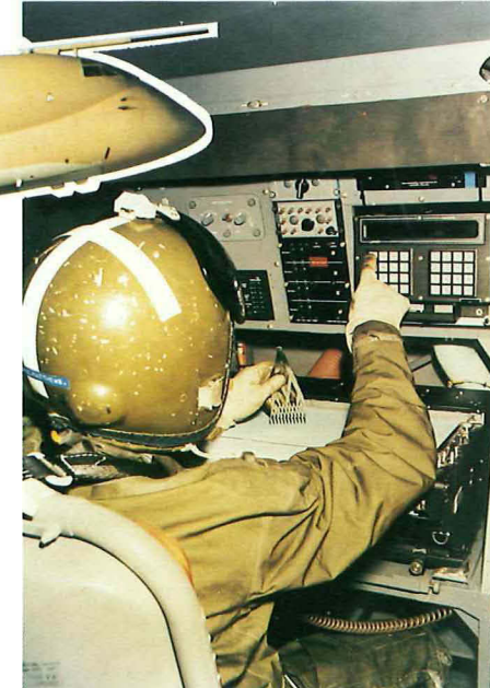
AQS902 Lightweight acoustic processing and display system, LAPADS, is in service on Royal Navy Sea King Mk 5 helicopters. This system can operate with free sonobuoys, or dipping sonar.
