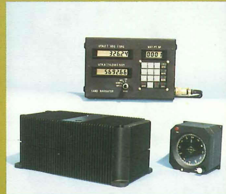
MAVLANS "strapdown" system for land navigation and gun control gives high performance at a fraction of alternative system costs.
