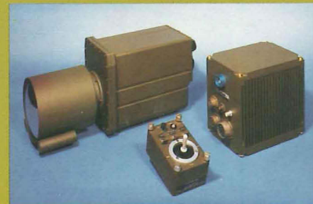
Indirect-view (Class II) imagers configured from Thermal Imaging Common Modules (TICM II) are widely used on land.
