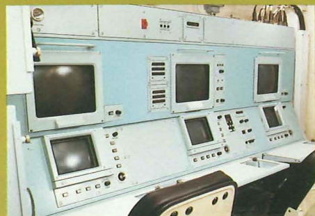
Shipborne processing and display systems for ship and submarine sonars, in service with the Royal Navy, are micro-processor based with touch operated control and display consoles.
