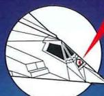
**2 SEEING IN THE DARK:** The 'Stealth' fighter detects its targets via the Forward Looking Infra-Red turret, or FLIR, embedded in its nose. This can provide a good picture of the target from several kilometres' range on even the darkest of nights.
