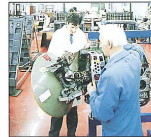
A Blue Parrot radar for the Buccaneer aircraft undergoing inspection prior to modification to update the radar for the Royal Air Force.
