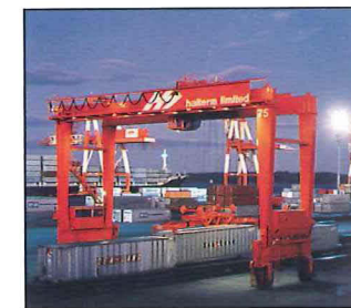
Ferranti Kairitainer diesel/electric rubber tyred gantry crane, Halifax, Nova Scotia, Canada.
